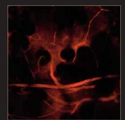
Excitation wavelength: 785nm Peak emission wavelength: 832nm Objective lens: CFI Plan Apochromat λ 20x
