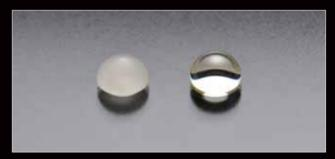
The front lens, which is the lens element at the tip of a high-power objective, is extremely small and has a distinctive shape. A highly skilled expert must grind the lens by hand to meet the required high-precision standards and desired shape. The ground lens is then stringently and repeatedly checked using high-precision processing technology to ensure it meets Nikon's compulsory high performance.
